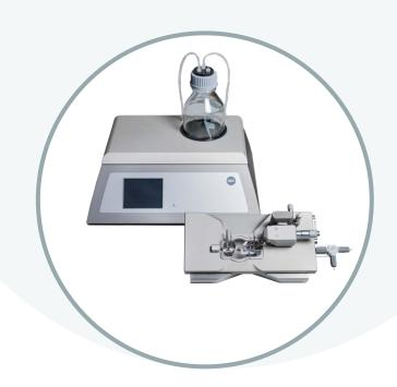
The Blind Sac Pressure or Perfusion Myograph System - 114PB is a system used to study the structure and function of isolated sections of small vessels (diameter >40  $\mu$ m) under near-physiological conditions. Vessel diameters can be measured in response to pharmacological and physiological stimuli.
