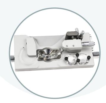
The Pressure or Perfusion Myograph System – 112PP is a system used to study the structure and function of isolated sections of small vessels (diameter >40 µm) under near physiological conditions.
