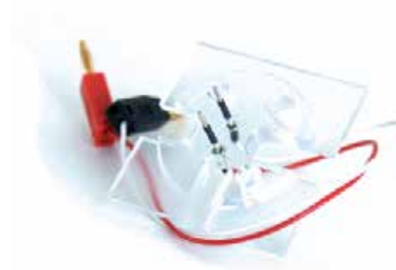
Figure 2.4 Chamber cover with built-in electrodes (optional item)
