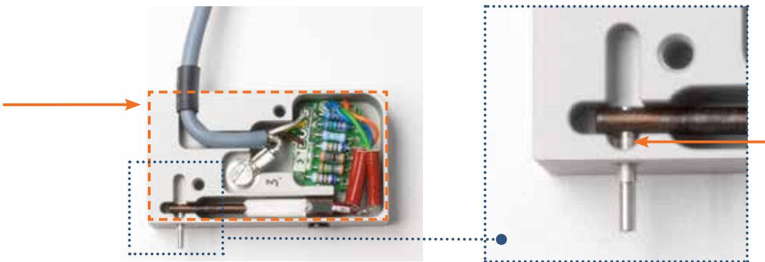
Figure 4.7 Inside the transducer housing and close-up of transducer pin.
