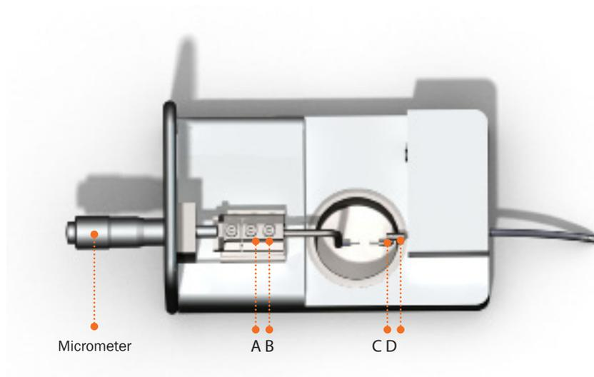
Figure 2.1 *Illustration of the screws for changing supports and adjustment of the pins*
