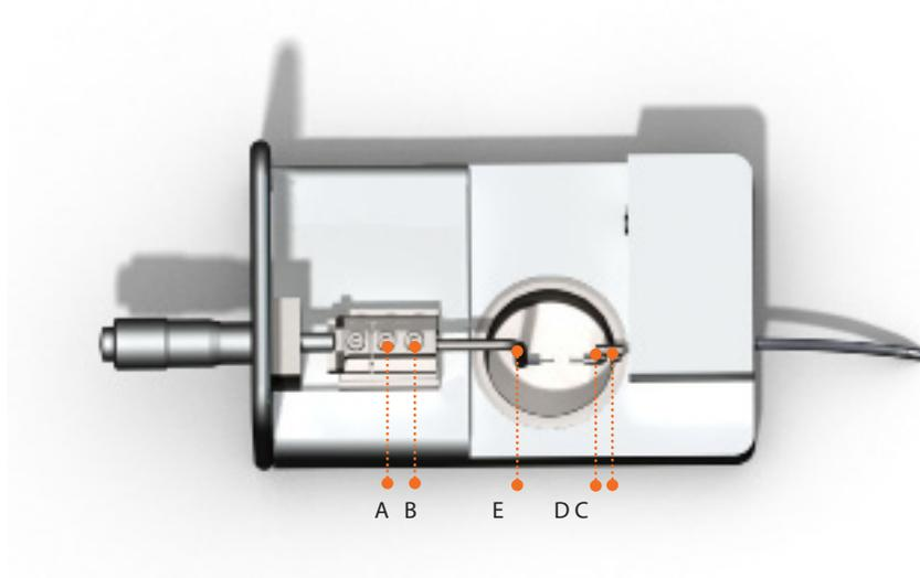
Figure 2.2 - Illustration of the screws for fine adjustment of the pins
