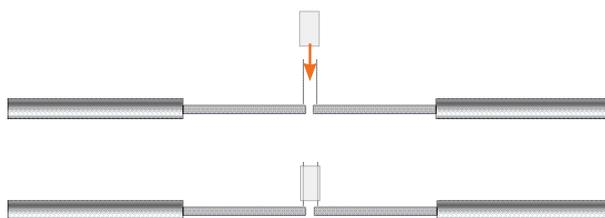
5. Slowly move the pins apart using the micrometer until the force reading is increasing.
