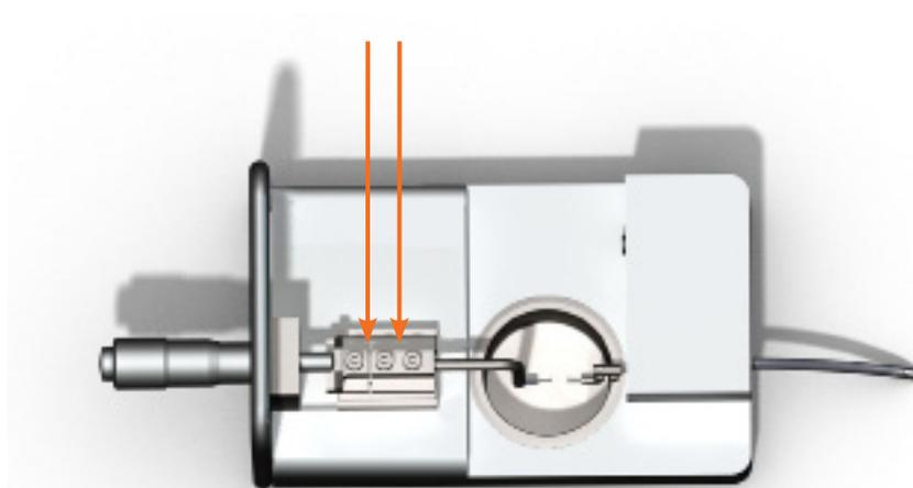
Figure 4.4 The areas where linear slide grease may be applied for smooth micropositioner movement
