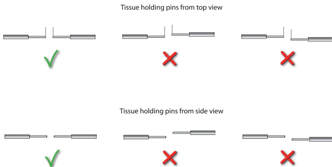
Figure 2.3 - Illustrations of properly aligned tissue holding pins (depicted on the far left) and incorrectly aligned pins (depicted in the middle and far right).
