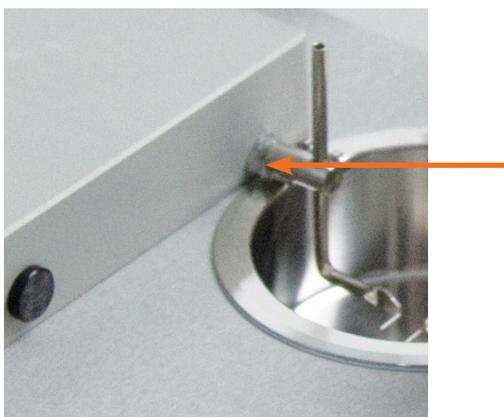
Figure 4.1 Close-up of transducer pin from outside.
