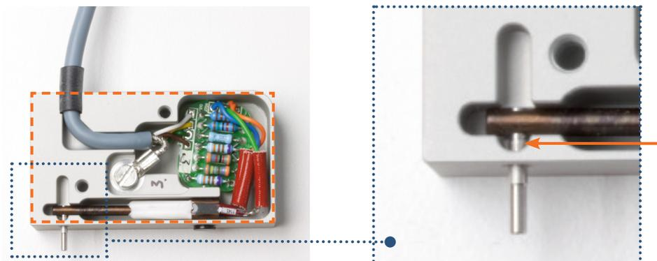
Figure 4.3 Inside the transducer housing and close-up of transducer pin.
