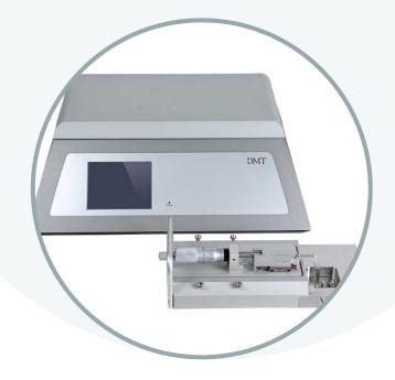
The Single Wire Myograph System - 320A is ideal for studying a single vessel with a diameter of 30 µm - 3 mm. The vessel is mounted as a ring preparation by threading it over two parallel stainless steel wires and securing the wires to two supports or "jaws". One support is attached to a precision micrometer, allowing manual control of vessel circumference and stretch. The other support is attached to a force transducer for measurements of force/tension development.
