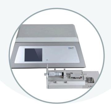
The Single Wire Myograph System - 320A is ideal for studying a single vessel with a diameter of 30  $\mu$ m - 3 mm. The vessel is mounted as a ring preparation by threading it over two parallel stainless steel wires and securing the wires to two supports or "jaws". One support is attached to a precision micrometer, allowing manual control of vessel circumference and stretch. The other support is attached to a force transducer for measurements of force/tension development.
