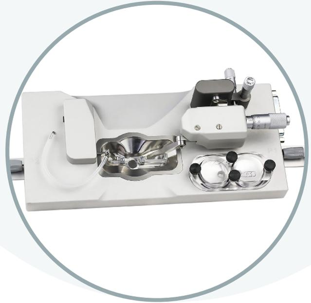
The Pressure or Perfusion Myograph System – 112PP is a system used to study the structure and function of isolated sections of small vessels (diameter  $>40 \mu\text{m}$ ) under near physiological conditions.
