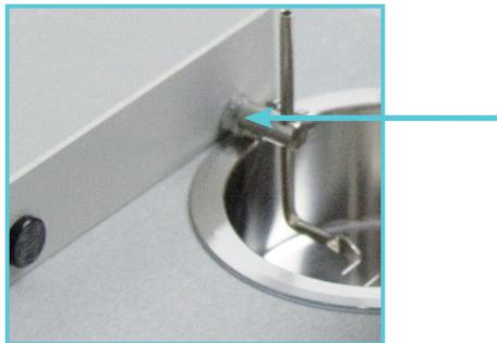
*Figure 4.1 Close-up of transducer pin from outside.*
