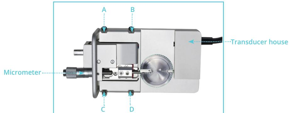
Figure 2.4 - Fine adjustments of the pins in the Myograph chamber
