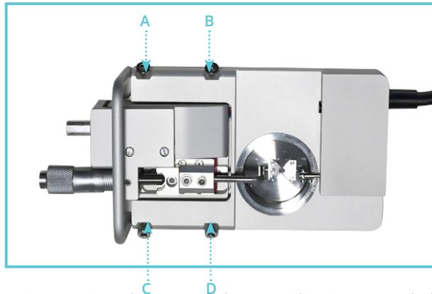
Figure 2.2 Fine adjustments of the jaws in the Wire Myograph chamber
