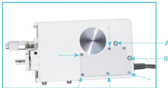
Figure 4.3 - The 8 screws that secure the transducer house to the chamber
