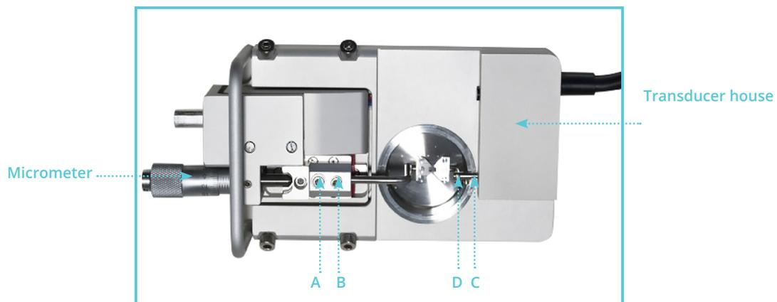
Figure 2.1 Illustration of the screws for changing supports and coarse adjustment of the jaws
