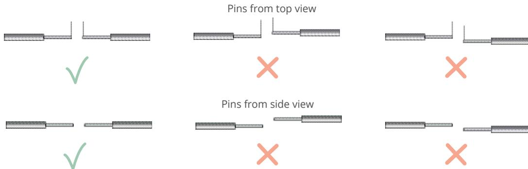
Figure 2.5 - Illustrations of properly aligned pins (depicted on the far left) and incorrectly aligned pins (depicted in the middle and far right).
