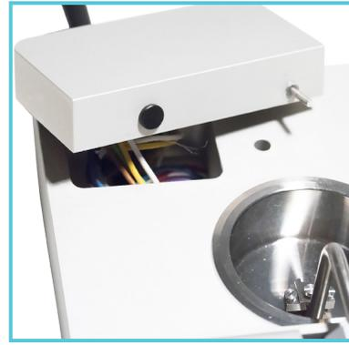
*Figure 4.4 Inside the transducer housing and close-up of transducer pin.*
