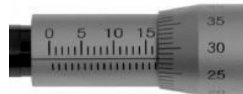
Figure A2.3 Example 2: reading = 16780 \mu\text{m}
