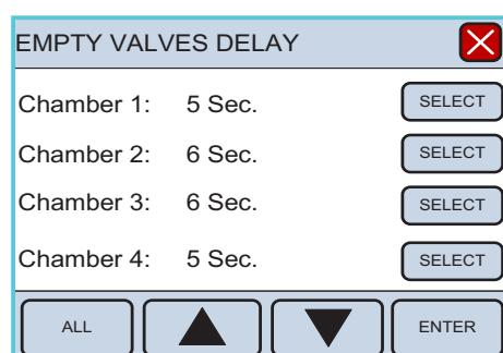
Pressing "ALL" will cause all the lines to turn blue, meaning all chambers can be modified at the same time. Again, the up and down arrow keys can be used to modify the length of time the vacuum valves stay open.
