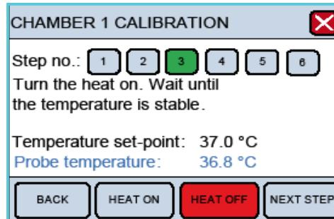
Covering the chambers with the chamber covers will expedite the chamber heating. Place the temperature probe into the chamber for the first calibration to monitor when the chamber has reached the target temperature. Heating will take about 20 to 30 minutes for the chambers and transducers to come to 37°C with the chamber covers in place. Once the chamber(s) are heated and have reached the target temperature, press "NEXT STEP".
