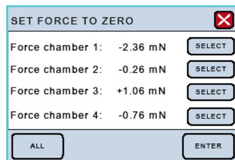
The line to be modified will turn blue, indicating that the interface is waiting for input. When "ALL" is chosen, all lines corresponding to all 4 channels will turn blue. Changing the numeric value for the chosen parameter can be done by touching the up or down arrow keys.
