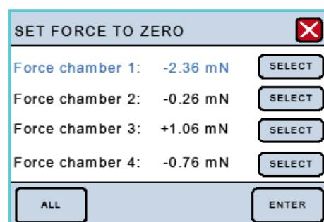
Once the desired setting has been chosen, pressing "ENTER" will lock the selection and be stored in memory. Pressing the white "X" in the red box will exit that menu and take you automatically to the Actual Force Display.
