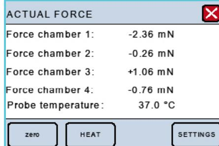
At any given time, if the force applied on any channel is out of range, the force reading for the overloaded channel will turn yellow as a warning.
