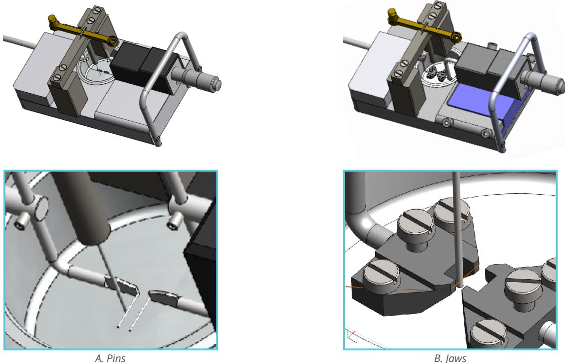
Figure 4.7 - Illustration of the proper placement for the balance transducer arm for calibration
