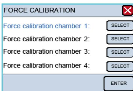
*Step 1* involves setting up the chamber for calibration. Make sure the chamber contains the pins or jaws, depending on the type of vessel being studied. If jaws are being used for smaller vessels, a wire needs to be strung on the transducer-side jaw for the calibration. Fill the chamber with double-distilled water for the volume to be used experimentally. Press "NEXT STEP".
