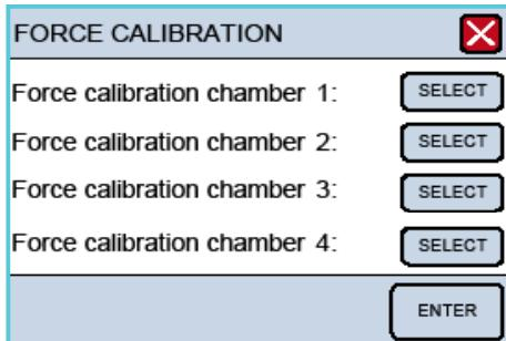
To begin the calibration, press "SELECT" for the chamber which calibration will be performed on. The text for the chamber to be calibrated will turn blue. Pressing "ENTER" will enter the 6-step procedure for calibrating the force transducer on the desired chamber.
