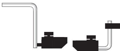
Figure 1.5 Mounting jaws for small vessels
