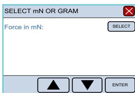
When the wanted force unit is shown press ENTER to select this force unit. The color of the text will turn black when it is saved in the system.
