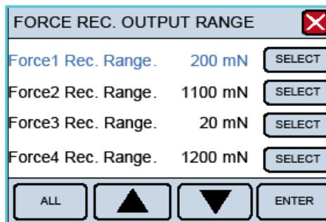
The "ALL" functions are used to change all four chambers Force Rec Output values at the same time. Pressing "ENTER" will store the numbers in memory for future experiments.
