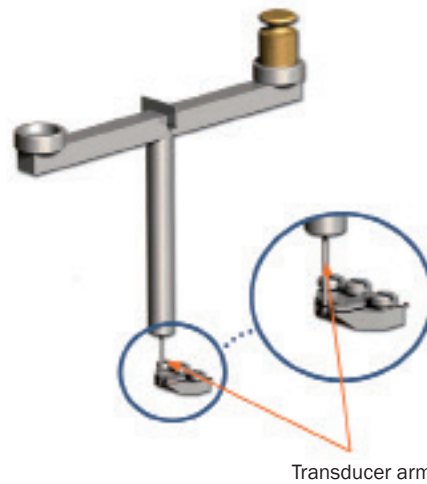
Figure 4.7 - Illustration of the proper placement for the balance transducer arm for calibration
