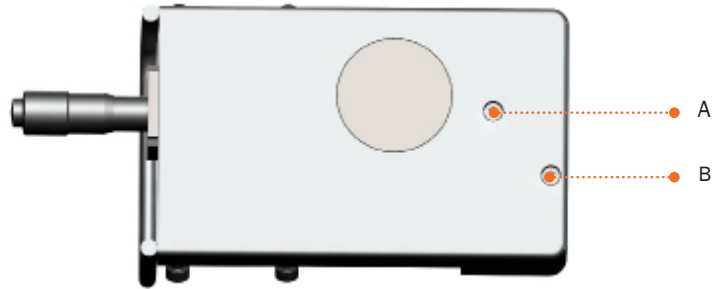
Figure 4.9 - The 2 screws that secure the transducer house to the chamber
